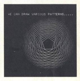
GRAPHIX performs essential tasks simply and efficiently — plotting points, drawing lines, displaying text and so on. X, Y co-ordinates are used to specify points — the bottom left-hand corner of the screen is the origin. The X-axis ranges from 0 to 319, the Y-axis from 9 to 199.
