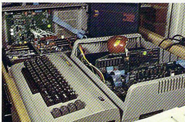
Top: inside the Spartan, with the CPU and Apple drive cards installed. The 1541 shows the custom DOS card installed.
