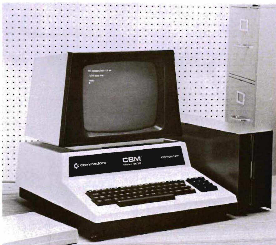
FIGURE 3—PEDISK II with 8" Disk Drive
