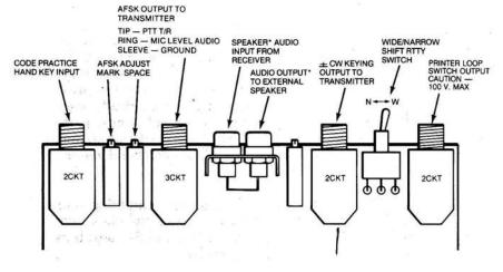
\*BOTH "SPEAKER AUDIO" PHONO JACKS ARE JUMPERED TOGETHER, SO EITHER CAN BE USED FOR INPUT-OUTPUT CONNECTIONS.
