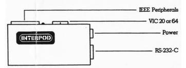
The computer may be connected to either of the 6 pin din sockets. The remaining socket allows additional IEEE serial peripherals such as the 1541 disk drive to be connected to the system. Many such devices may be connected to Interpod by the usual chaining method.
